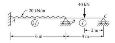
5. Determine the reaction components for the propped cantilever subjected to UDL as shown in figure?
